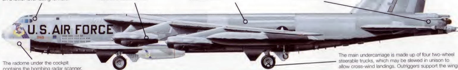
B-52s carry an enormous amount of fuel – around 147,112 litres (38,863 US gal) – in large internal tanks in the fuselage and wings. The J57-powered models also carry water tanks for the water injection system used by the engines during take-off to increase thrust.
